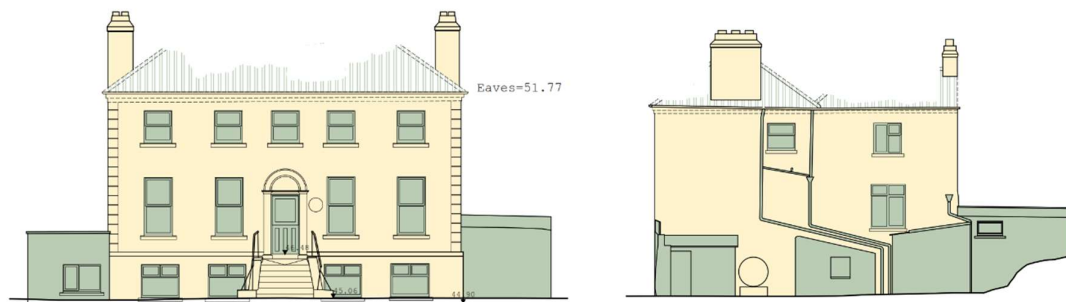
Fig 7: Front (L) and north (R) Existing elevation, historic fabric in yellow, modern in green
