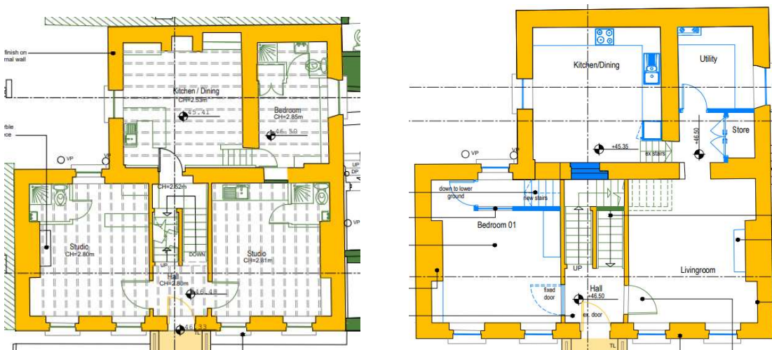
Fig 18: Existing Entrance Plan (L), Proposed Entrance Floor Plan (R), Historical Fabric (Yellow), Modern Retained (Green), Proposed (blue)
