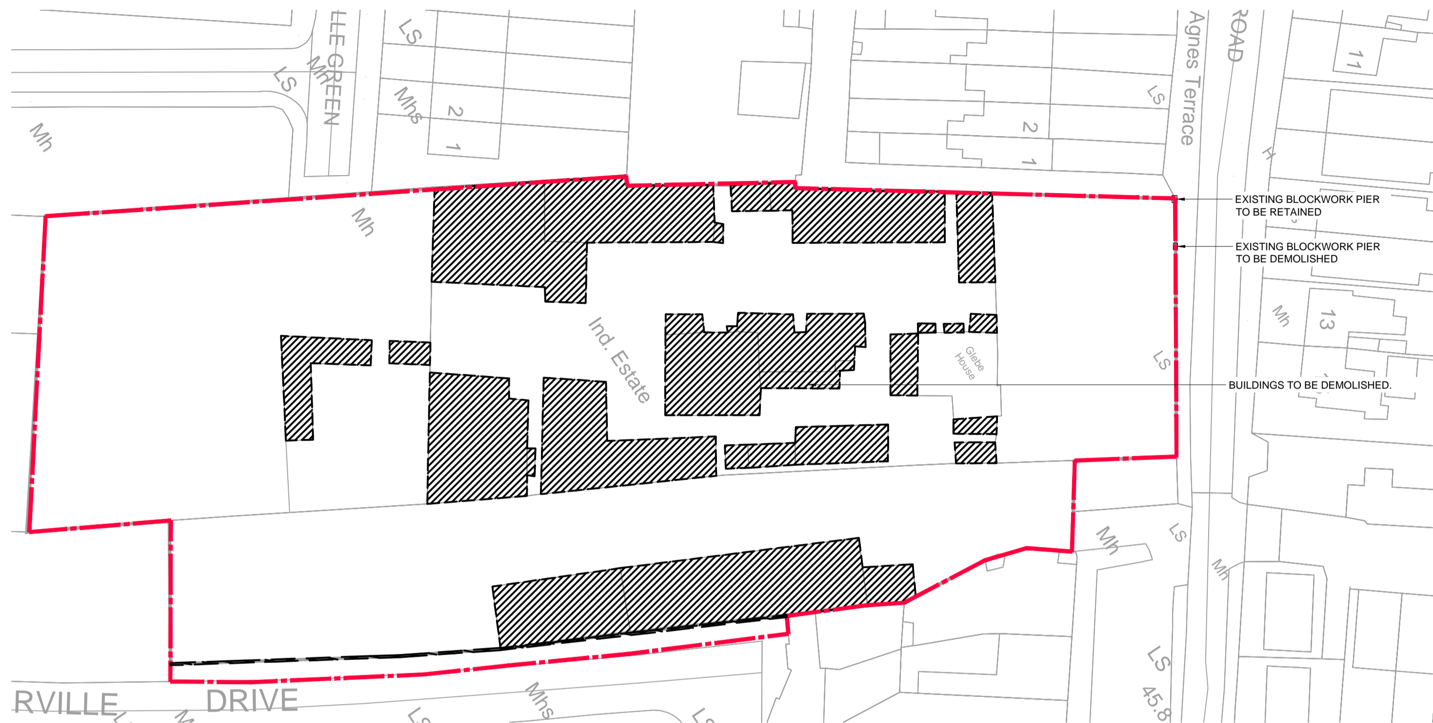
STAGE 1 - DEMOLITION PLAN SCALE 1:500
